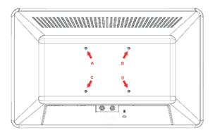
Use the four holes (A), (B), (C), and (D) to attach the swing arm or other mounting fixture to the back of the monitor with screws (not supplied).
